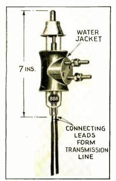
Fig. A. The unusually small size of this water-cooled, high-frequency triode tube can be realized when an ordinary I kw. transmitting tube is 2 to 3 ft. high. When employed as an oscillator this tube may be operated at its maximum power rating on frequencies as high as 240 mc.; while in amplifier circuits, where the input and output circuits are isolated, it may be run to full output on frequencies as high as 300 mc. (I meter). The power output as oscillator on 100 mc. (3 meters) exceeds 700 W.
